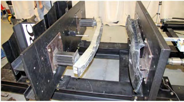
**Figure 13.** The impact bars for the bumpers in System C after QS C1. The Sedona's impact bar fractured at the center and around the mounting brackets.
