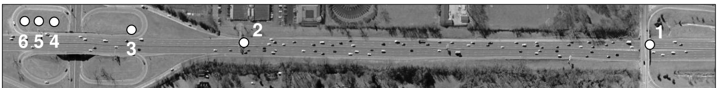
Figure 9. Aerial image of the crash site of the GMC Yukon Denali rollover. The six vehicle positions used to calculate the translational velocity of the vehicle are indicated with white circles and numbered.
