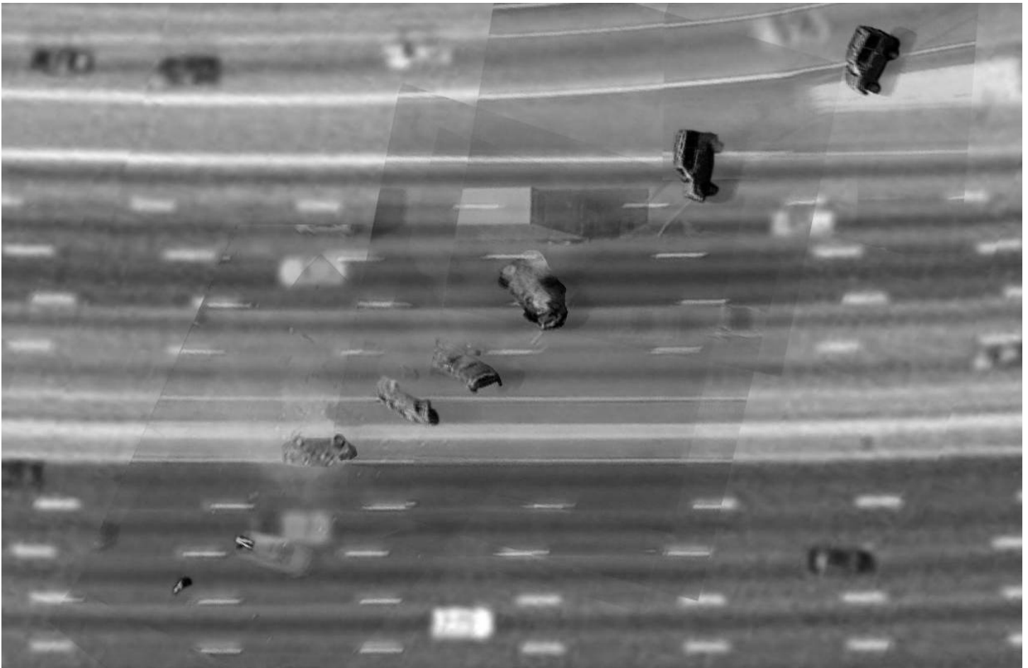
Figure 4. Rectified video images from the Lincoln Navigator rollover overlaid on an aerial photograph. Key vehicle and occupant positions have been highlighted.
