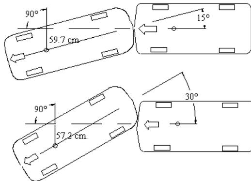
Fig. 6 – Test Configuration: 15 & 30 degrees
