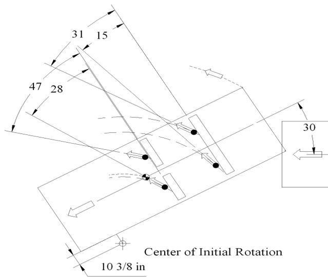
Fig. 11 -Variations of Force Direction in Degrees by Seat Position
