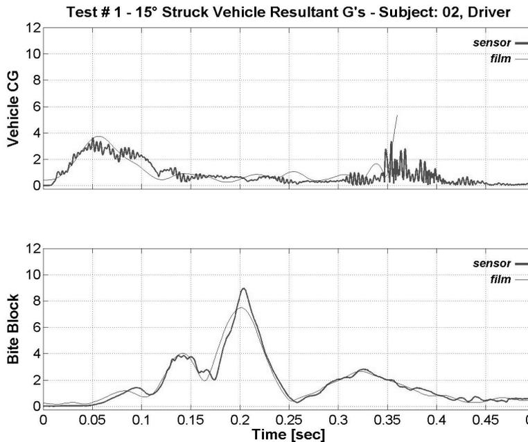
Fig. 7 – Comparison of Motion Analysis and Sensor Data
