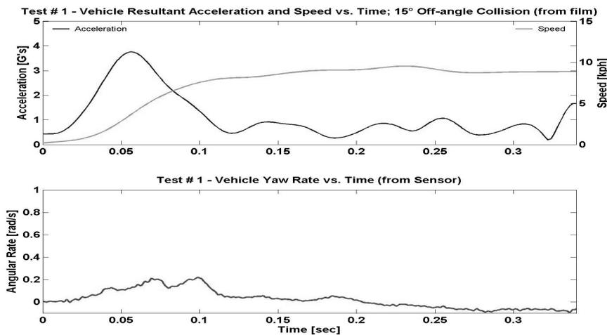
Fig. 8 - 15<sup>0</sup> Impact: Struck Vehicle Resultant Acceleration/Velocity Change
