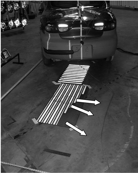
Fig. 10 - 30 degree impact: Right Rear Tire Track (Arrows)
