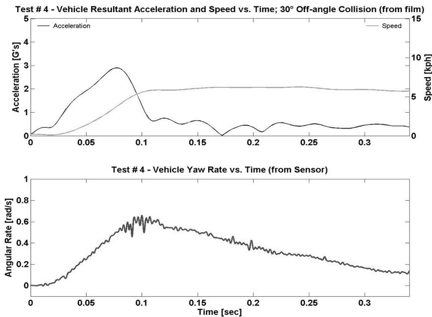
Fig. 9 – 30<sup>0</sup> struck Vehicle Resultant Acceleration/Velocity Change
