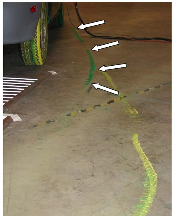
Figure 14 – 30° test, right-front tire track (Arrows).
